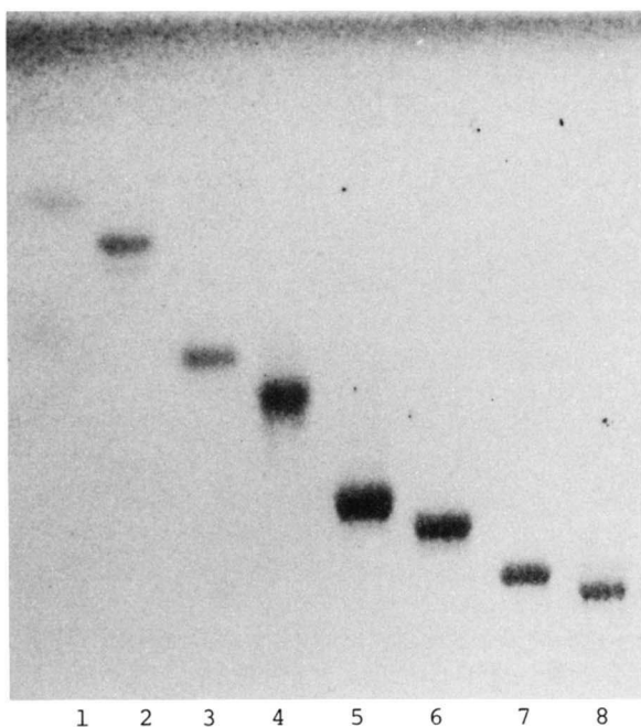
Fig. 1. Thin-layer chromatogram of isolated glycosphingolipids. Lane 1, GL 1b with nonhydroxy fatty acid; 2, GL 1b with hydroxy fatty acid; 3, GL 2a with nonhydroxy fatty acid; 4, GL 2a with hydroxy fatty acid; 5, GL 3 with nonhydroxy fatty acid; 6, GL 3 enriched with hydroxy fatty acid; 7, GL 4 ; 8, GL 5 . GL 1b was obtained from bovine brain white matter. GL 2a , GL 3 , and GL 4 were obtained from hog erythrocyte membranes. GL 5 was obtained from sheep erythrocyte membranes. The plate was developed with a solvent system of chloroform–methanol–water 65:25:4 (by volume). Glycosphingolipids were visualized by anthrone sulfuric acid reagent.
